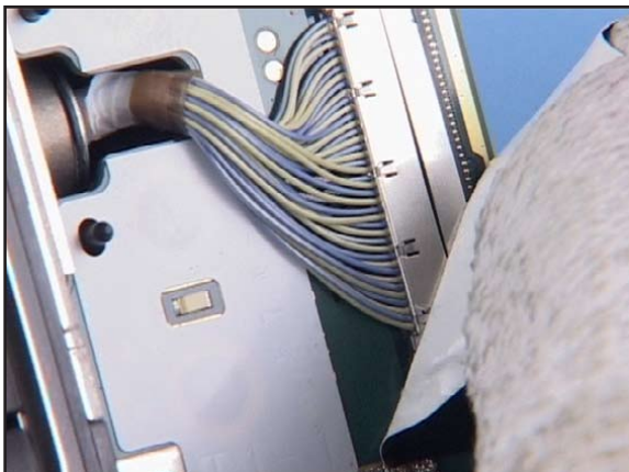
9. Peel up the COAX CABLE SUPPORT TAPE
