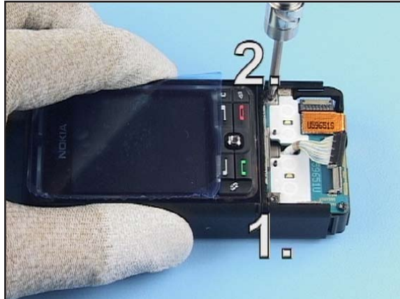
8. Apply the torque of 18Ncm to the screws in the order shown.
