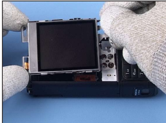
10. When the clips are released properly, the shield can be lifted up easily.
