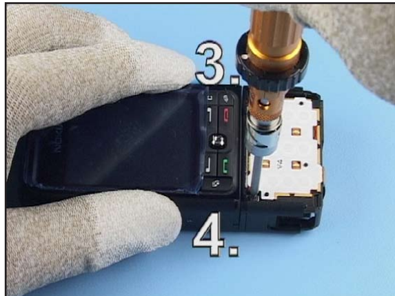
10. Continue tightening the next screws with the torque of 18 Ncm in the order shown.
