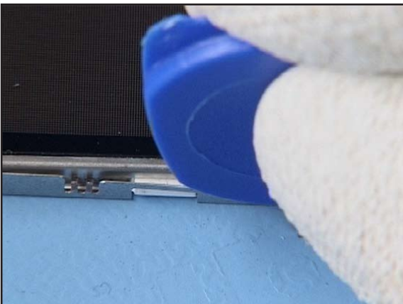
11. Separate the LCD MODULE by releasing the 4 snaps with the SRT-6.
