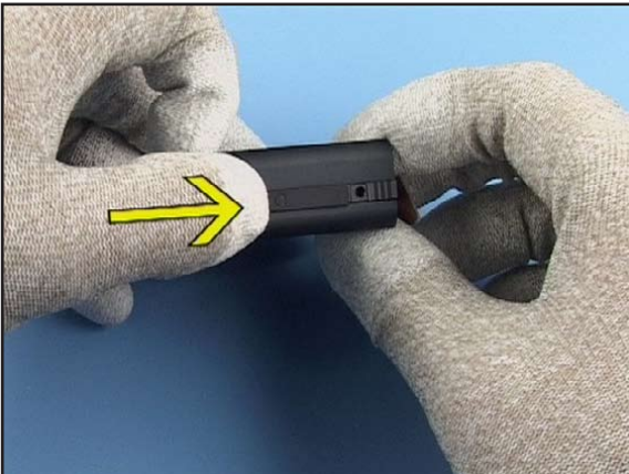
27. Shift out the MAIN FLEX ASSEMBLY and discard it. Do not use it again when assemble.
