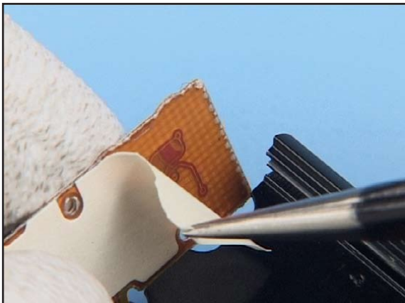
3. Peel up the cover tape from the DOMESHEET.
