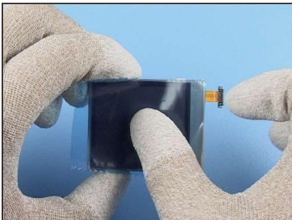
13. Cover the display with a protective film.
