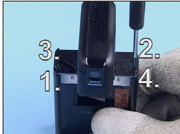
22. Unscrew the 4 screws in the order shown.
