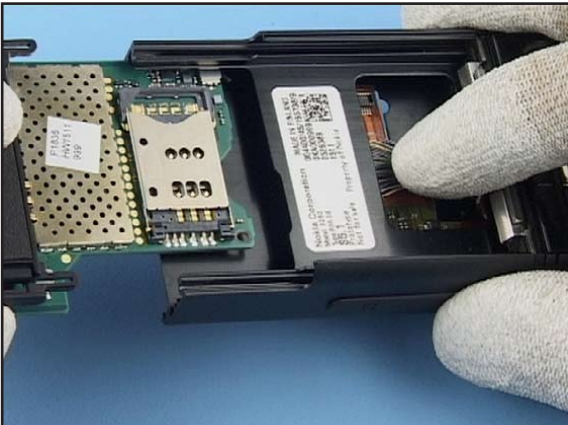
15. Push down the Cables while shifting the assembly into the UPPER FRAME ALUMINIUM.
