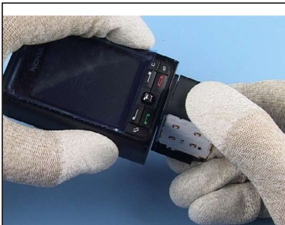
11. Turn the upper block in order to prevent mechanical stress to the joystick while unscrewing the screws.
