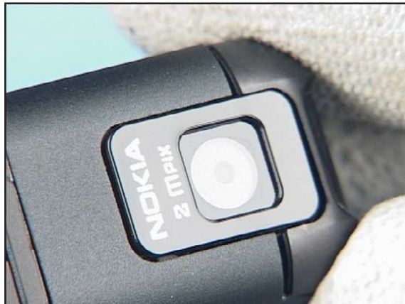
26. Check the window for correct positioning and cleanness.
