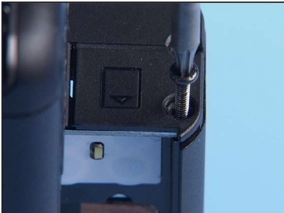
9. Tighten the 4 screws slightly.
