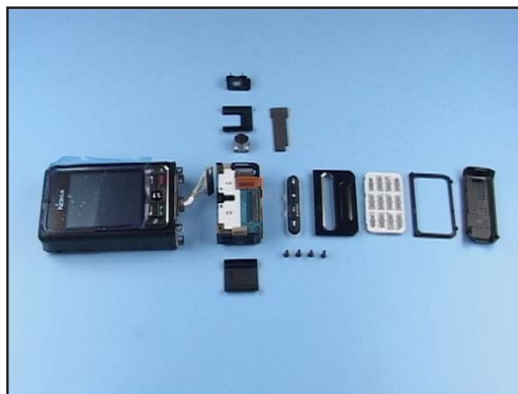
18. The disassembly procedure of the upper block is now completed.
